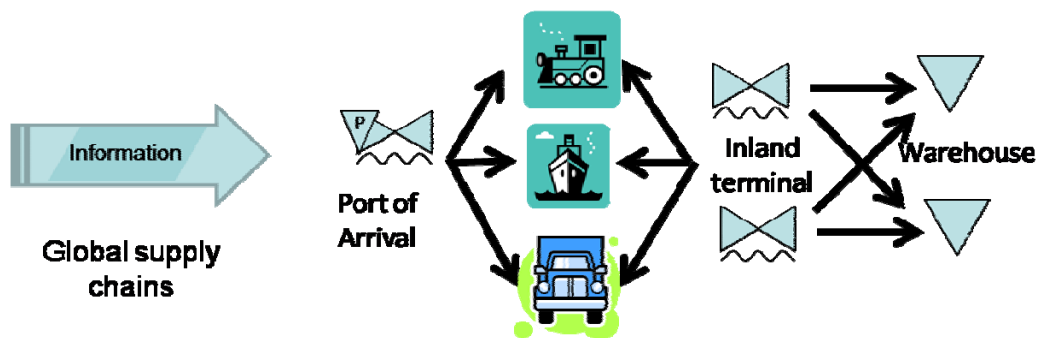
Figure 1.1. Sea port hinterland intermodal transport network
