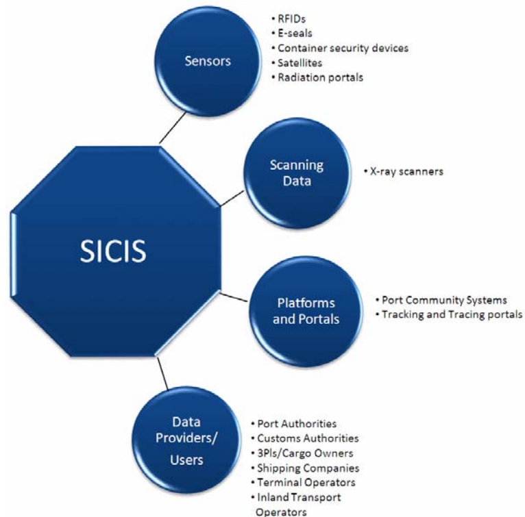
Figure 4. The Shared Intermodal Container Information System (SICIS) will process data from different data sources and communicate with various platforms
