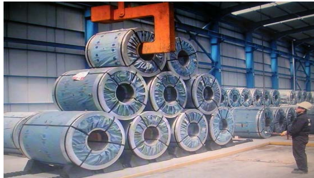
Figure 1. An example of pyramid stacking in warehouses.
